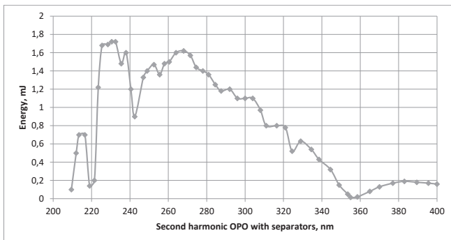
Typical tuning curve of second harmonic OPO
