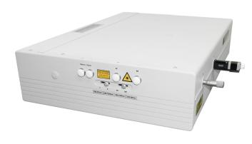
LS-2134-LT40 and LS-2145-LT50 are fully integrated laser systems that combine Q-switched pump laser and Ti sapphire converter of Nd:YAG second harmonic radiation (532 nm) into tunable near IR, UV and visible spectral band. They are designed for scientific research in photochemistry, biology, medicine, for PAT and LIBS applications. The lasers consist of laser head, power supply (PS), cooling system (CS) with water-to-air heat exchanger, controller (CU) and remote control (RC).
